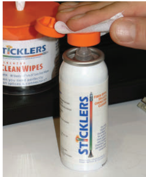
Pictured here is a technician wetting a wipe with an appropriate cleaning fluid.
